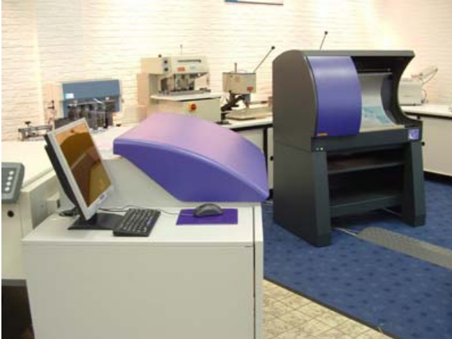
A modern CTP system. Plates are now made without using film.
