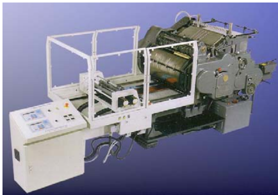
Metallic Foil is applied using this hot-stamping conversion to a Heidelberg cylinder press
