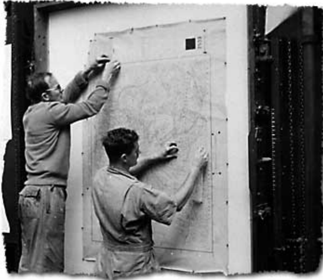
Compilation of a map on the copyboard before reproduction
